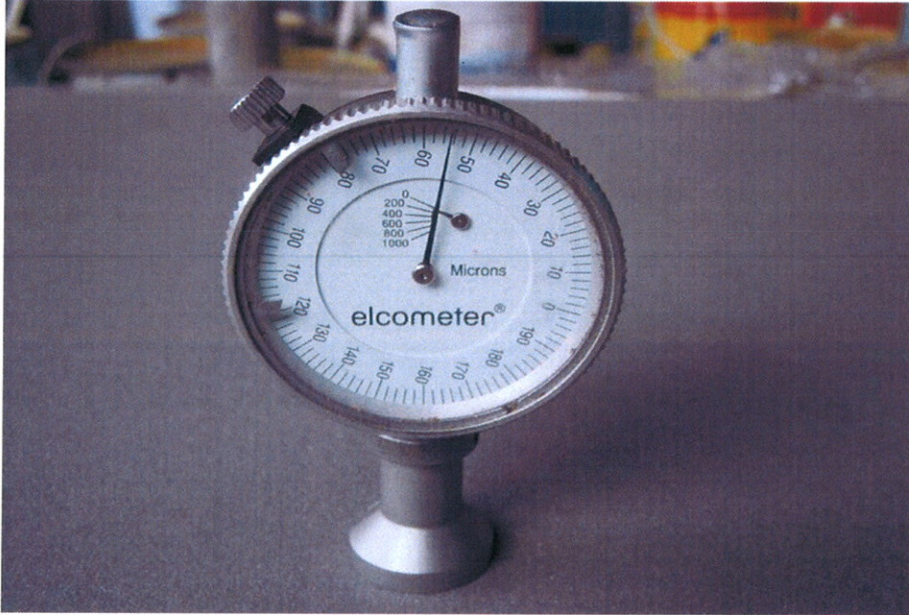
1. Photo shown the surface profile reading taken was 55 microns.
